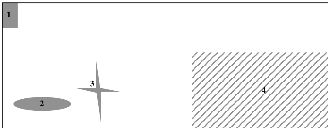
Fig. 1.4. Possible shapes of failure regions, represented here as grey areas in a two-dimensional section of a program's demand space. Analysis of actual defects in programs [Bishop et al. 1986, Ammann & Knight 1988, Bishop & Pullen 1988, Hatton & Roberts 1994] has shown that they may produce failure regions with simple shapes like 1 and 2 in this picture, but also complex "stars" or "snowflakes" or even non-connected regions like region 4 here.
